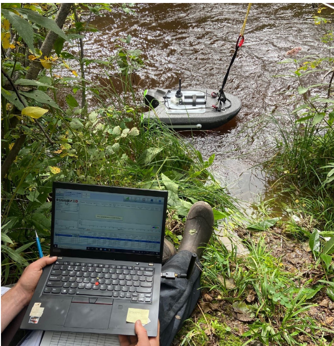
Flow monitoring station with ADCP boat
