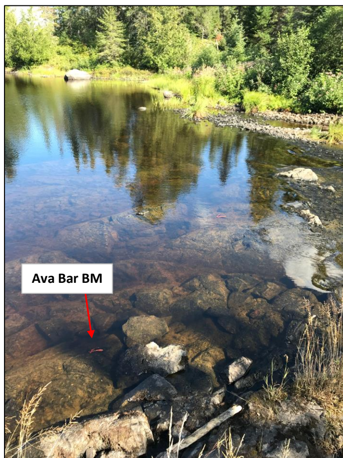
Photo B1. Position of Ava iron bar used for water level measurements at Ava Lake.
