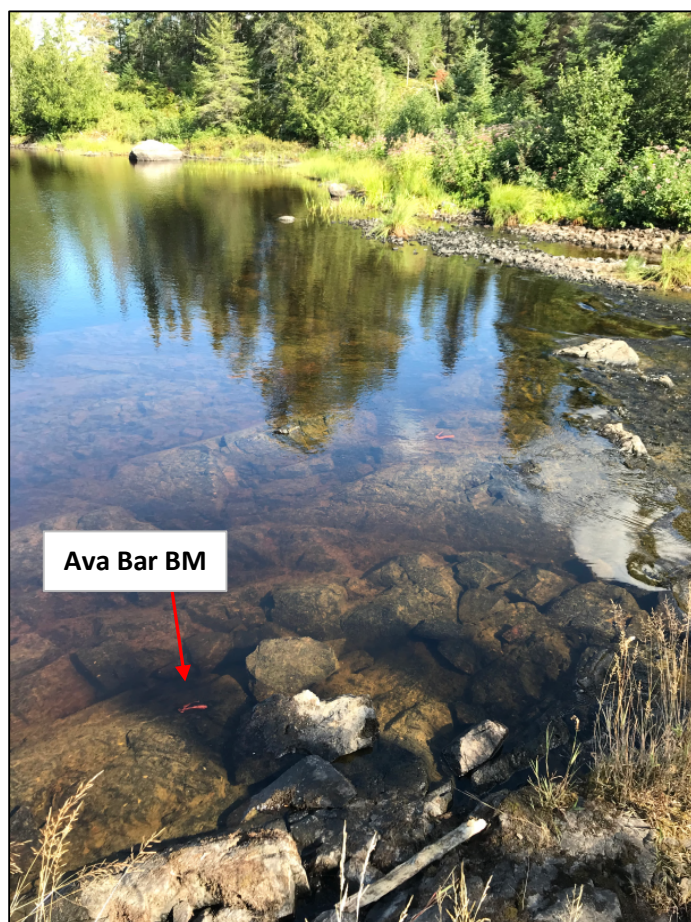
Photo B3 Position of Ava iron bar used for water level measurements at Ava Lake
